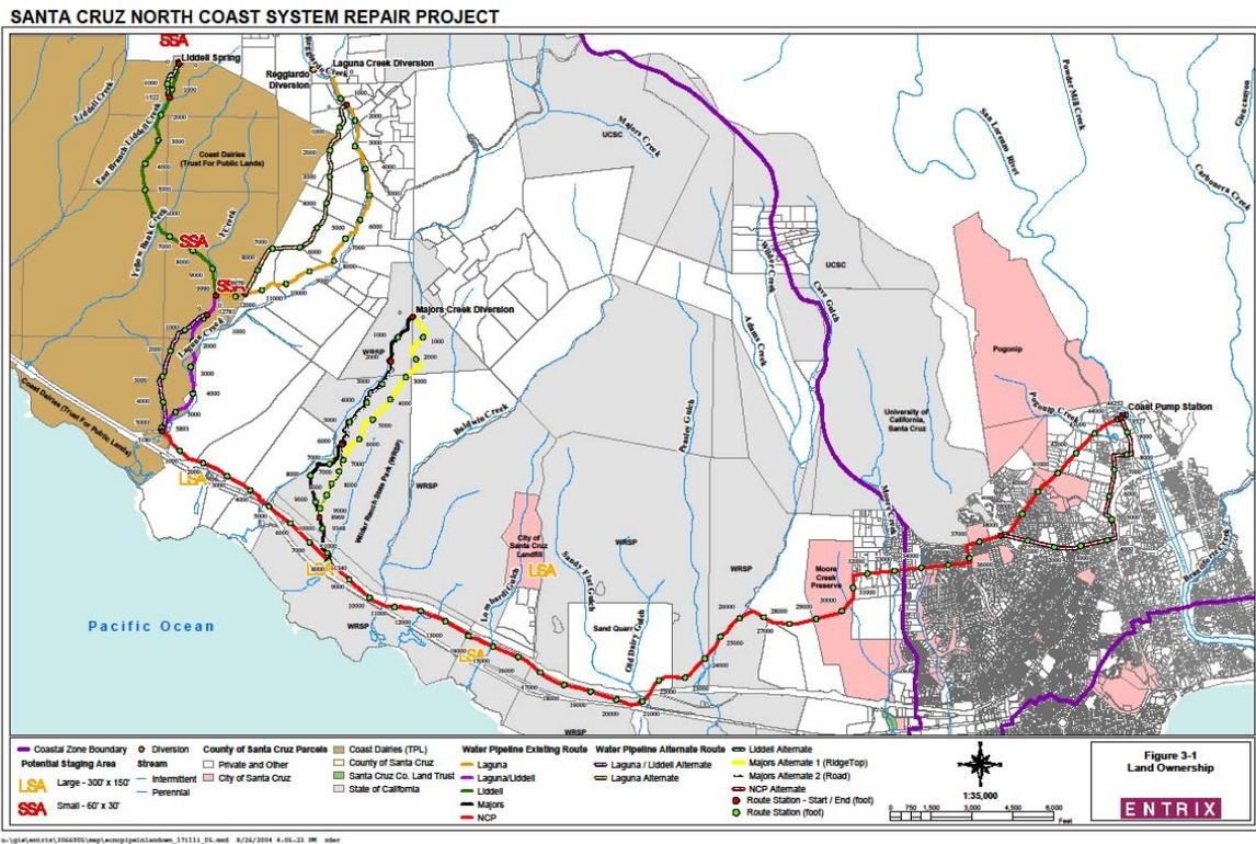
The 9-mile long, 50-year old **Newell Creek Pipeline** delivers raw water from Loch Lomond Reservoir through Henry Cowell State Park to the GHWTP. The age and condition of the pipe, coupled with the environmental conditions through which the pipeline was installed, require that portions of this pipeline
