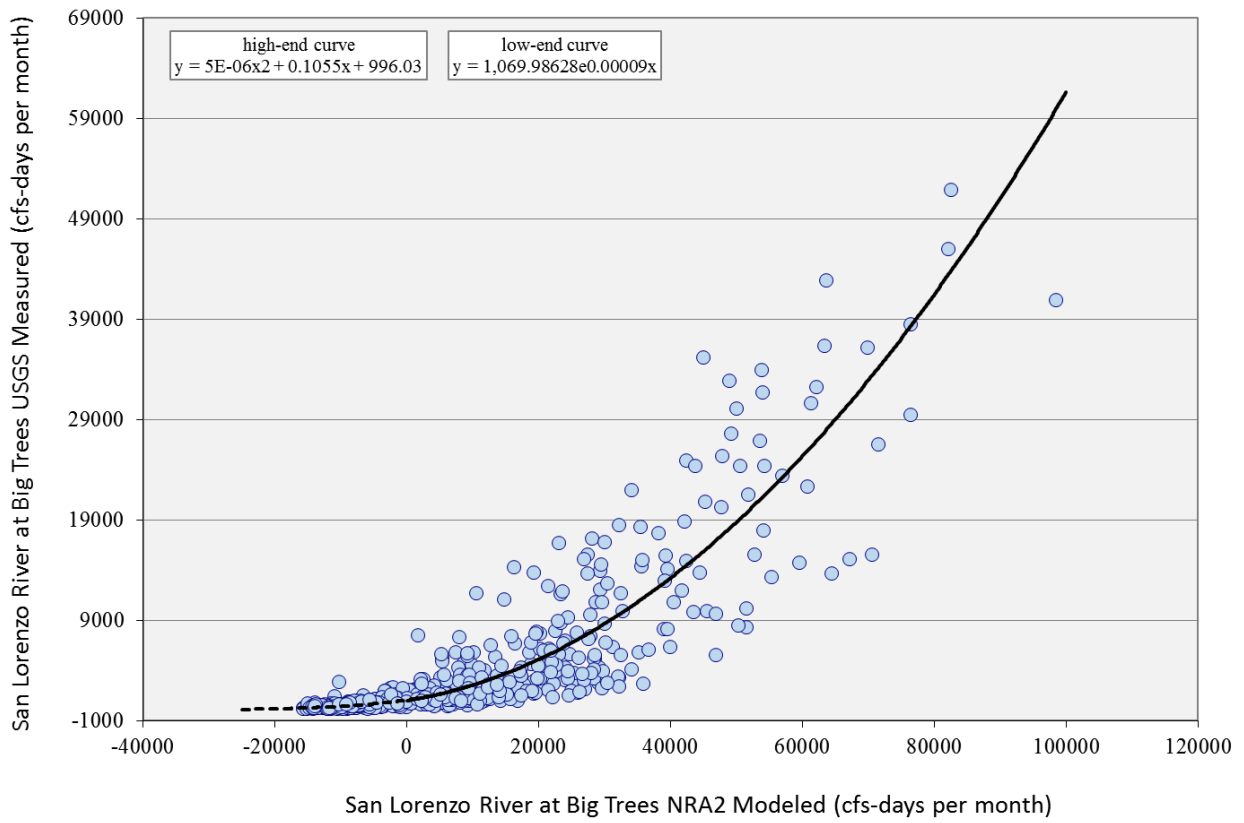
Figure 2: Calibration curve between monthly streamflow at Big Trees computed with
