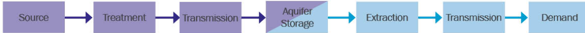
SCHEMATIC OVERVIEW - KEY COMPONENTS FOR CA-10 WATER REUSE FOR AQUIFIER RECHARGE IPR
